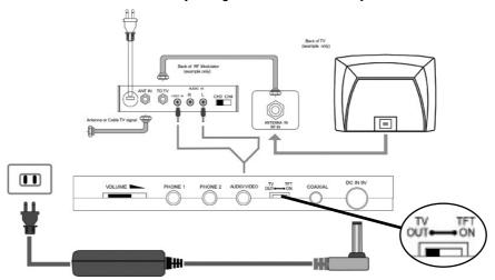
Before you begin, make sure you have an RF modulator and extra RF coaxial cables. These are not supplied with the player, but are available from Magnavox or most consumer electronics retailers.
